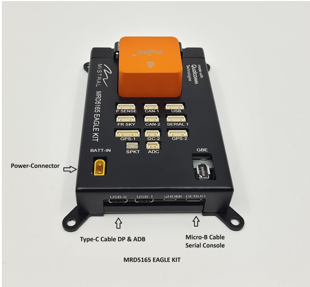
Figure 4 MRD5165 EAGLE KIT HOST PC Connectors
