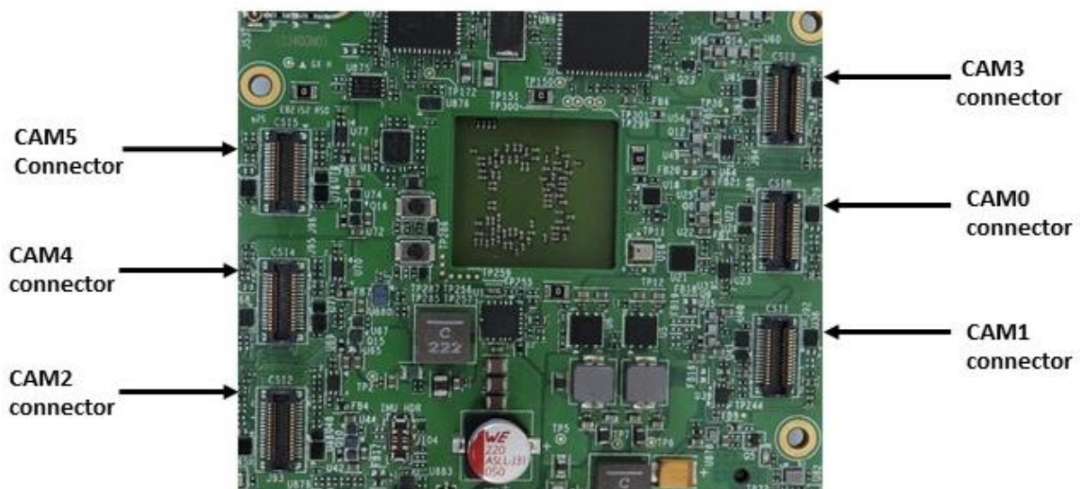
Figure 5-1: MRD5165 Eagle Board Camera Connectors
