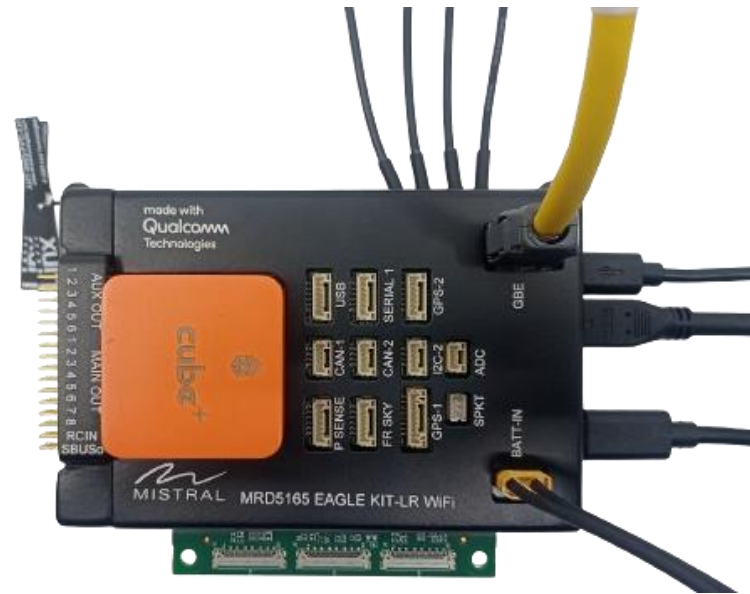
Figure 8-1: MRD5165 Eagle Kit LR Wi-Fi - System setup
